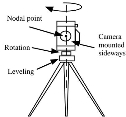
Figure 8. Camera setup for taking overlapping pictures.
