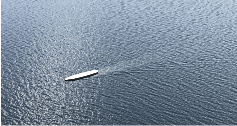
Figure 3.4: Kelvin wake and turbulent wake generated with the ocean toolkit.
