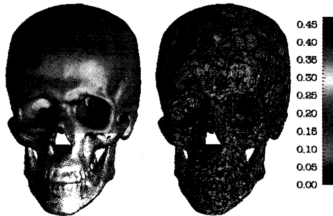
15 Simplified skull (a) mesh and (b) color-coded approximation errors in pixel units—with aggressive border straightening: \epsilon = 4.0 (2.55 percent of original triangles).
