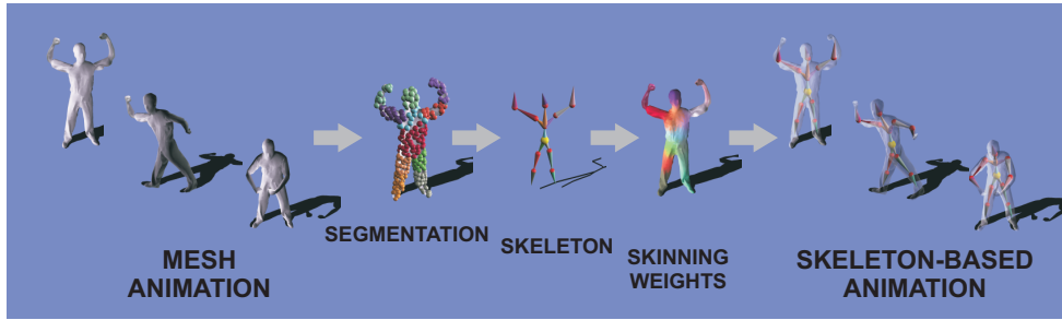
Figure 2: Overview of our algorithm: using an animated mesh as input, our approach segments the model into plausible approximately rigid surface patches (shown in different colors), estimates the kinematic skeleton (joints shown in red) and its motion parameters, and calculates the skinning weights connecting the skeleton to the mesh. The output is a skeleton-based version of the input mesh animation.
