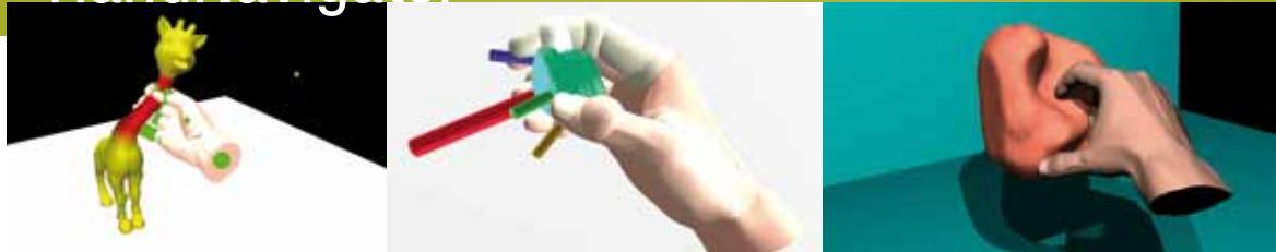
The HandNavigator is designed to control a virtual hand using 10 or more degrees of freedom with high accuracy.
