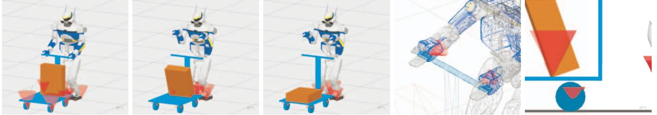
Fig. 4. HRP-2 pushing a cart, then lifting it up and finally releasing it (the last two snapshots show contact points at hands and box).
