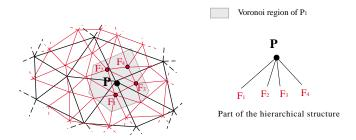
Figure 6: A hierarchical structure is built by connecting each node of a given LOD to the nodes of the next LOD that are included into its Voronoi region. These children will replace  $P_1$  if sampling becomes too coarse
