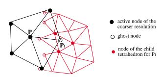
Figure 4: Ghost nodes are used for enabling the joint use of different LODs during simulations (2D view, coarse mesh is black, finer mesh is grey).
