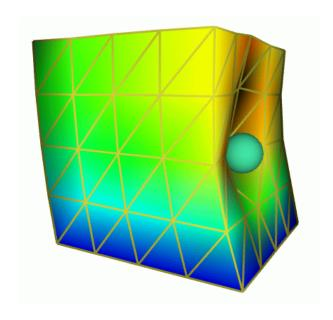
Figure 7: The cube's down face is fixed. With  $\mu=10^6$ , the volume preservation creates an intuitive deformation when the sphere is pulled inside the cube.
