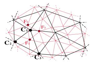
Figure 5: Linking the LOD meshes (2D drawing): node  $C_1$  will pull information from finer level using its child element  $(F_1, F_2, F_3)$ . Information can also be pushed to node  $F_1$  from its parent element  $(C_1, C_2, C_3)$ , depending on which level is actually simulated.
