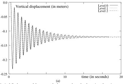
Vertical displacement of the corner of a I meter cube under the action of gravity with damping. Three different resolutions are plotted. Physical coefficients are  $\lambda=40,000$  and  $\mu=100,000$ .
