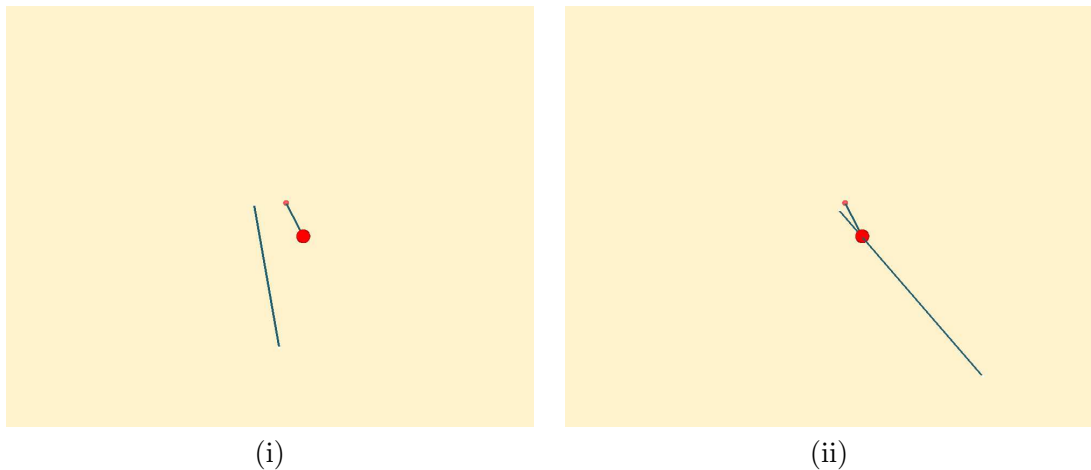
Fig. 4.16: Continuous collision detection between two moving coplanar edges.
