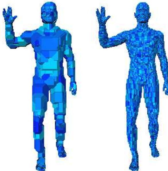
Fig. 2.5: Two levels of an 18-DOP hierarchy [MKE03].
