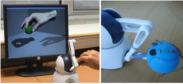
Figure 2: Our first prototype (left) and the second (right), augmenting the Phantom stylus with pressure sensors and a soft ball that serves as a proxy for the virtual objects to be grasped.
